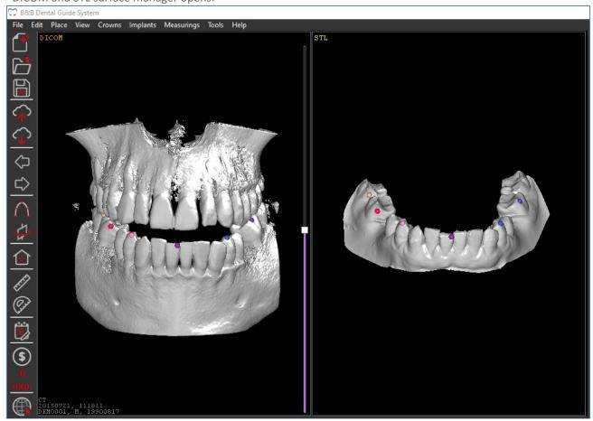
The next step is to place identical dots (red, green, blue etc.) on the DICOM file surface and in the same sequence on the STL surface. Pressing the "ALIGN" button closes the combining manager and the STL surface is placed in the project in the specified position. After automatic alignment, you may need to adjust in manual mode.
