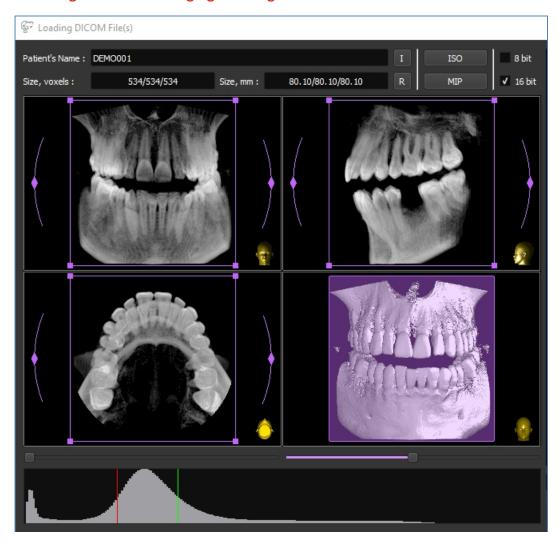
In the DICOM alignment and slices range selection (DICOM cutting) window set the desired range of slices by moving the window borders. To do this, place mouse pointer over the border of the window in projection of interest, drag and drop it in the corresponding direction, holding the left mouse button. Rotate the volume by dragging\* the pointer, located on the semicircles around the corresponding projection.
